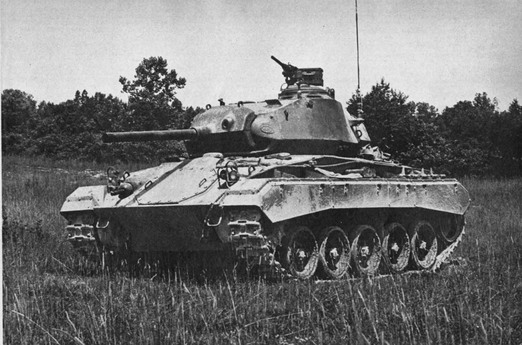
WITH A 75-MM. GUN, M-24 OUTCLASSES OTHER LIGHT TANKS IN ARMAMENT. NEARLY AS FAST AS THE M-5A1, IT IS LONGER, WIDER AND HEAVIER
